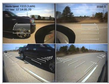
Video VBOX 4 camera system used to test Blind Spot Detection
